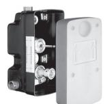
Remove the upper styro-foam cover from the tap body, attach the assembling plate and insert the threaded rods into the CF through the holes marked No. 2 on the assembling plate and screw the ø5 mm threaded rods (2pcs) into the CF. Secure the assembling plate to the concealed tap using the securing nuts.
