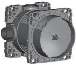
Unscrew the two plugs from the CF with a No. 8 Allen wrench, then screw in the  $\frac{1}{2}$ " AL plugs with M4 thread in their place. Place the assembling plate with the corresponding holes onto the securing (guide) points of the tap body. Screw the M4 threaded rods through the assembling board into the threads in the plugs. Secure the assembling plate to the CF using the M4 securing nuts.
